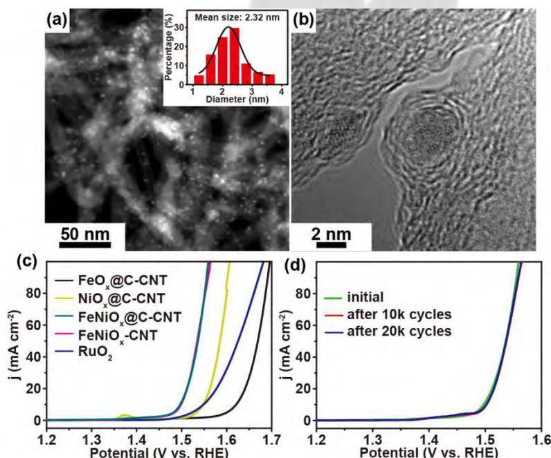
Figure 1. (a) HAADF-STEM image and (b) HRTEM image of FeNiO<sub>x</sub>@C-CNT, (c) the LSV curves of corresponding catalysts with iR-compensation measured in 1 M KOH at a scan rate of 5 mV s<sup>-1</sup>, (d) LSV curves of FeNiO<sub>x</sub>@C-CNT before and after stability test.
