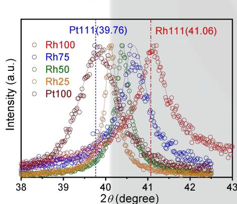
Figure 1 XRD profiles of NPs fabricated in RhPt mixed solutions.
