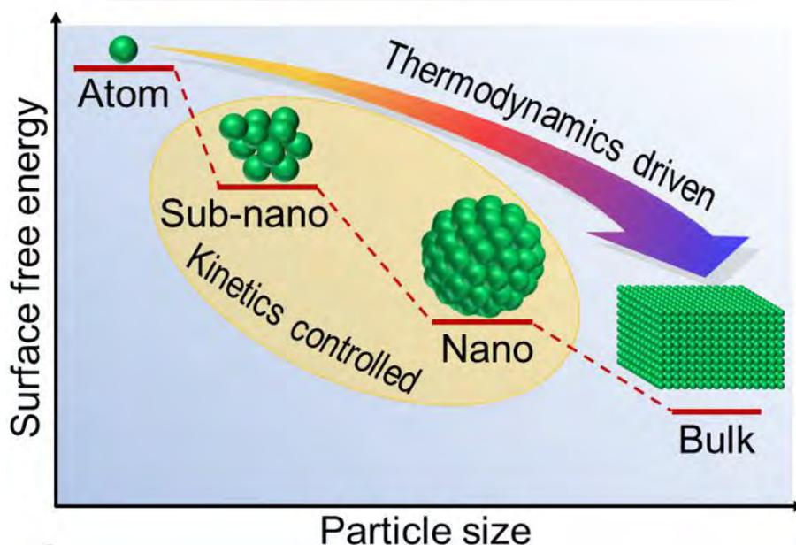
**Figure 1.** Kinetics dominated evolution of metal particles under pulsed high-temperature.
