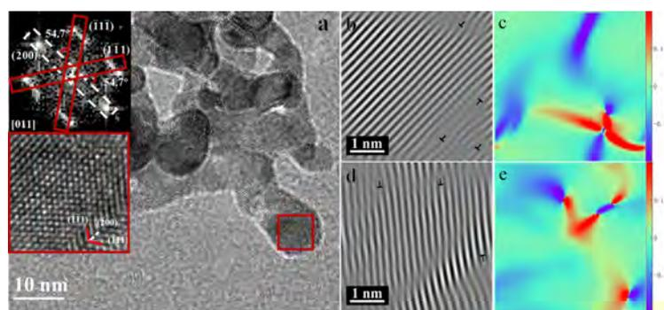
Figure 2. The defect and strain characterizations of the L-Pd aerogel. (a) HRTEM image of the L-Pd aerogel. The insets are the enlarged image and Fourier transform image of the red frame area in (a). (b,d) IFFT patterns of  $(\bar{2}00)$  and  $(1\bar{1}1)$  planes, respectively. (c,e) Strain distributions of the  $(\bar{2}00)$  and  $(1\bar{1}1)$  planes, respectively. (The positive and negative values on the scale bar represent tensile and compressive strain)
