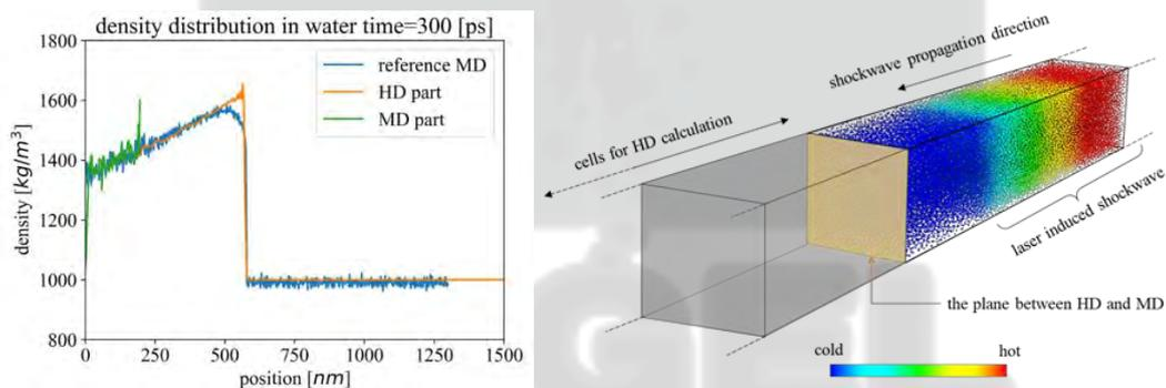
**Figure 1.** (a) Density distribution predicted for 300 ps after laser irradiation of a Ag target by a 10 ps laser pulse by a hybrid MD-HD simulation (orange and green curves) and a pure MD simulation with longer computational cell (blue curve). (b) Snapshot of an interfacial region between MD and HD parts of the model shown for a time before the shock wave reached the interface. The atoms in the MD region are colored by temperature and the orange plane is the boundary of MD domain.
