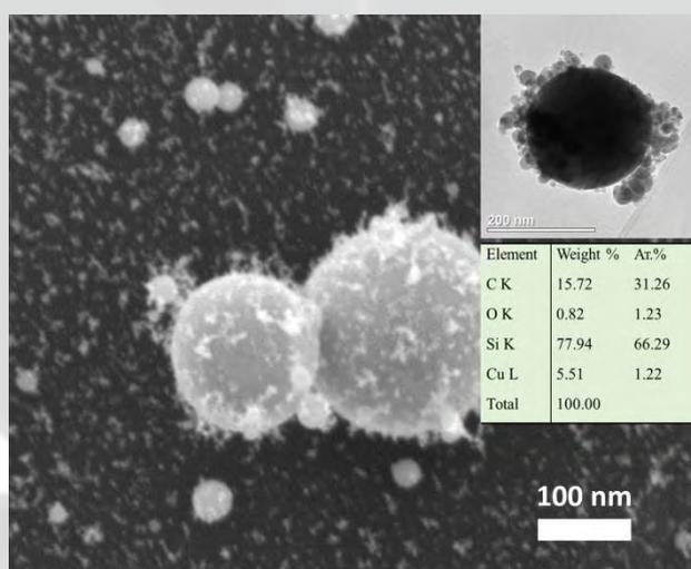
Figure 1 SEM image of Cu nanoparticles; insets: TEM image and EDX analysis
