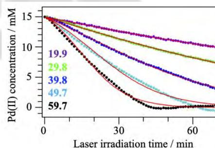
Figure 2 Temporal changes of the Pd(II) concentration in various laser fluences. Red lines are fitting curves of the kinetic model.
