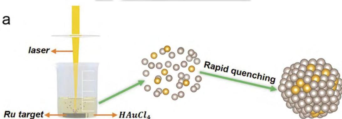
Figure 1 Schematic diagram of the synthetic process for single-atom catalysts.
