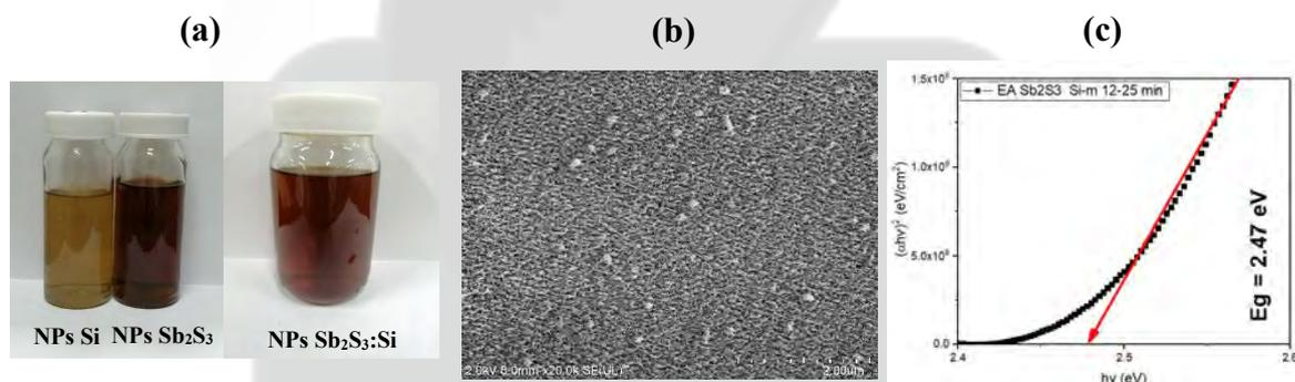
Figure 1 (a) Nanocolloids of  $\text{Sb}_2\text{S}_3$  and mono-Si by PLAL and their mix (b) Micrography of  $\text{Sb}_2\text{S}_3$  with mono-Si (c) Band gap  $\text{Sb}_2\text{S}_3$  with m-Si.
