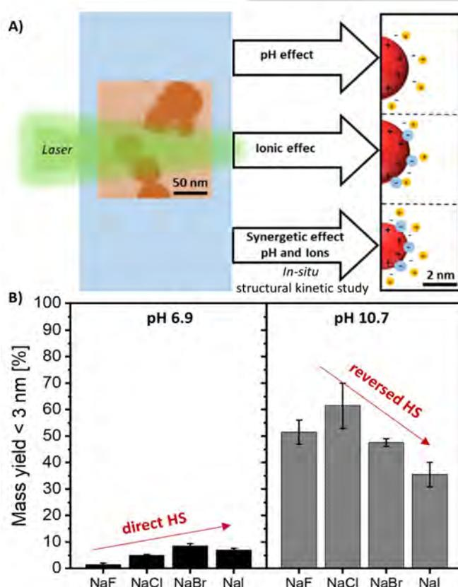
Figure 1 : A) Illustration of the fragmentation process, including visualisation of studied chemical influence factors [3]. B) Mass yield of particles after LFL using a 9 ns laser (532 nm, 0.1 kHz, 1.6 J/cm<sup>2</sup>) [3].
