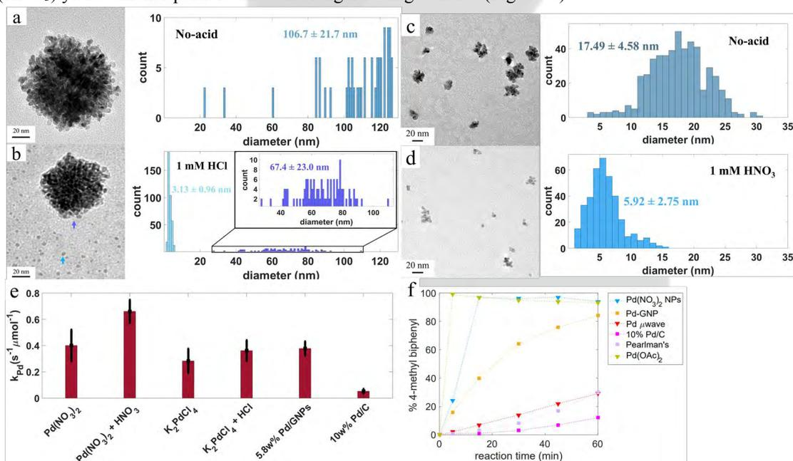
Figure 1. Representative TEM images with size distributions of PdNPs synthesized using K<sub>2</sub>PdCl<sub>4</sub> in (a) no acid and (b) 1 mM HCl, and Pd(NO<sub>3</sub>)<sub>2</sub> in (c) no acid and (d) 1 mM HNO<sub>3</sub>. (e)  $k_{Pd}$  values for laser-PdNPs and other Pd-based catalysts. (f) 4-methyl biphenyl formation over time in the presence of Pd catalysts.
