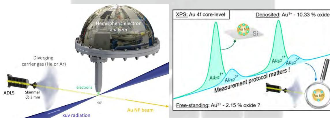
Figure 1 : (Left panel) Experimental setup of the XPS measurement of the Au NPs beam generated by means of the aerodynamics lens. (Right panel) Surface oxidation states of the Au NPs as a function of the measurement protocol.
