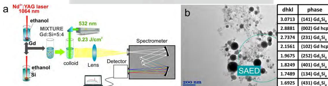
Figure 1 Schematic diagram of the experimental set-up (a) and results of characterization of the synthesized particles (b).
