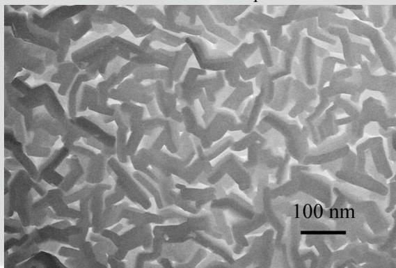
Fig. 1. NPs of Cu Pc at various stages of laser fragmentation after 10 min of fragmentation. Scale bar denotes 100 nm.
