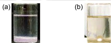
Figure.2 (a) CaO gel-AuNPs, and (b) CaO gel-PtNPs composite obtained by mixing a CaO gel colloid and a AuNP or PtNP colloid prepared by laser ablation in ethanol.
