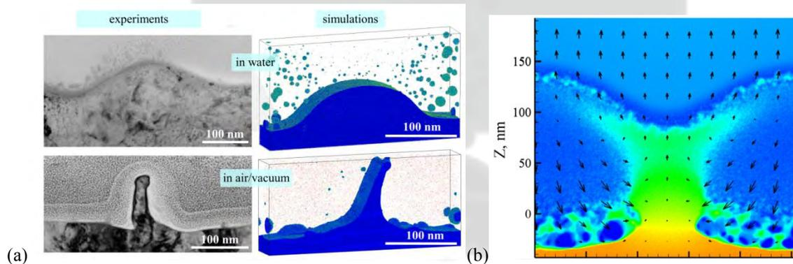
**Figure 1.** Results of experimental and computational study of the generation of surface morphology on a Cr (001) target irradiated by a single 200 fs pulse in water and vacuum/air: (a) The shapes of the surface protrusions observed in TEM images of cross-sectional slices extracted from irradiated spots and predicted in large-scale atomistic simulations; (b) Contour plot of density distribution predicted in the simulation for a time of 200 ps after the laser pulse.
