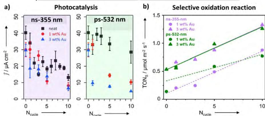
Figure 1: Effect of PuDEL of P25-TiO<sub>2</sub> (without and loaded with 1 wt% and 3 wt% of laser-generated Au NPs) on the catalytic activity shown for a): Photocurrent density  $j$  in photocatalysis<sup>[2,6]</sup> and b): Turn-over number (TONs) of ethanol to acetic acid during selective oxidation reaction<sup>[2]</sup>. Data are shown with respect to the number ( $N_{\text{cycle}}$ ) of laser irradiation cycles (–number of laser pulses) applied. Figure was taken from Ref. [2].
