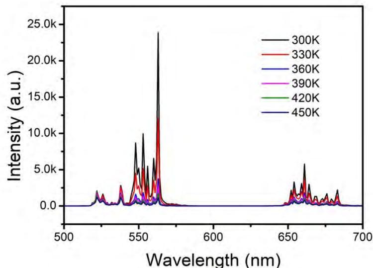
Figure 1 Upconversion photoluminescence spectra of products as a function of temperature
