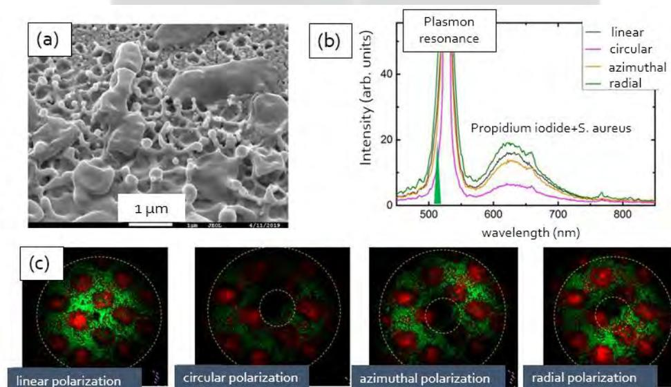
Figure 1. (a) SEM image of laser-fabricated nanopikes on a 1- $\mu\text{m}$  thick gold film; (b) photoluminescence spectra of bacteria on Au nanopikes, acquired at different polarization; (c) microphotographs of the dead (red) bacteria, illuminated with 515-nm laser radiation with the corresponding polarization.
