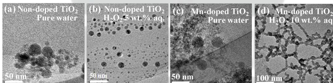
Figure 1 TEM images of TiO<sub>2</sub> nanoparticles synthesized by laser ablation in pure water and H<sub>2</sub>O<sub>2</sub> aqueous solutions: (a), (b) non-doped TiO<sub>2</sub>, (c), (d) 0.1 mol% Mn-doped TiO<sub>2</sub>.
