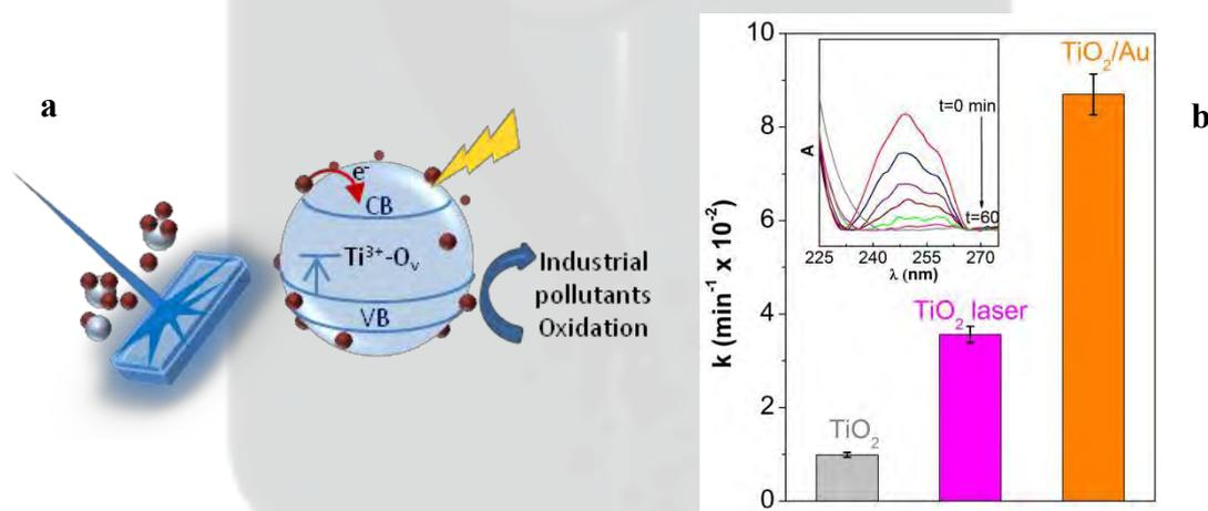
Figure 1 . a) Defects induced by laser irradiation on TiO<sub>2</sub>; b) kinetic constants of the photodegradation of the BTX/sulfolane aqueous solution, inset: UV-VIS spectra of the solution in presence of TiO<sub>2</sub> laser treated catalyst.
