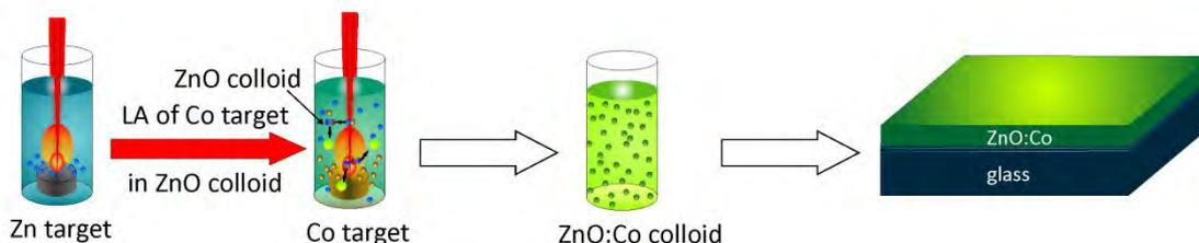
Figure 1 Schematic illustration of the experimental procedure used for preparation of cobalt-doped zinc oxide nanostructures
