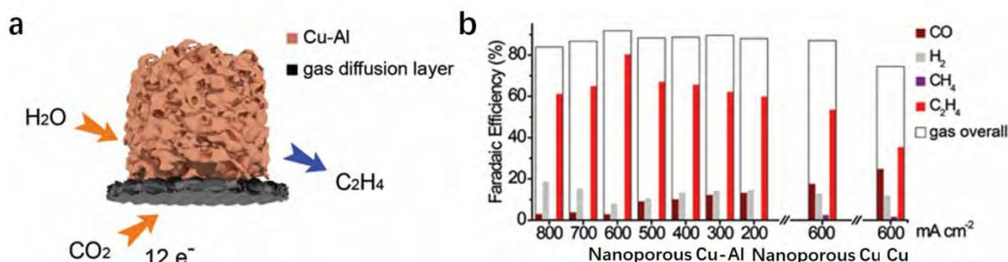
Figure 1. a. Schematic of electrochemical reduction of CO<sub>2</sub> to C<sub>2</sub>H<sub>4</sub> using the nanoporous Cu-Al catalyst on a gas diffusion electrode. (b) Electrochemical performance of CO<sub>2</sub> to C<sub>2</sub>H<sub>4</sub> with Cu-Al and Cu under different testing conditions.
