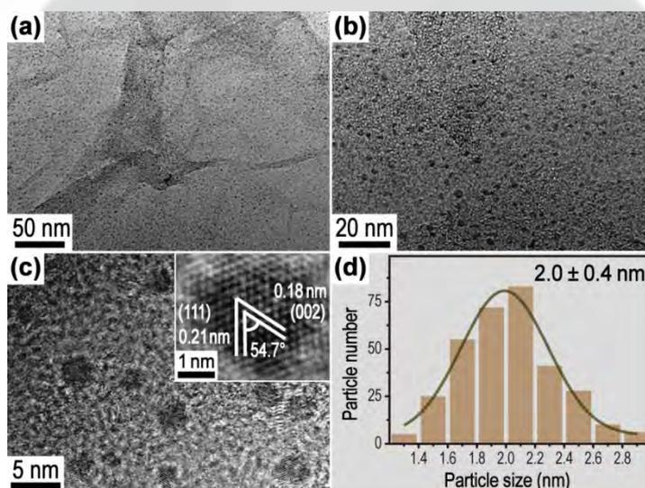
Figure. (a, b, c) TEM images of Cu/rGO NCs. (d) size distribution histogram of Cu NPs.
