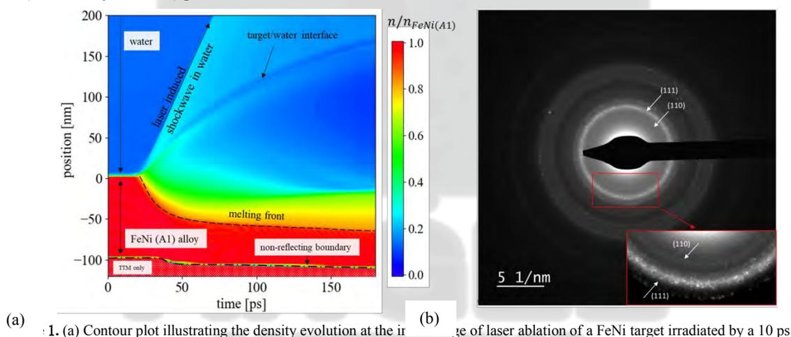
(a) Contour plot illustrating the density evolution at the interface of laser ablation of a FeNi target irradiated by a 10 ps laser pulse, as predicted in a large-scale atomistic-continuum simulation. (b) TEM/SAD diffraction pattern of FeNi nanoparticle, where the diffraction ring of plane (110) indicates the appearing of the superlattice structure.
