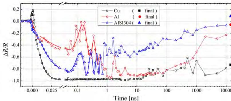
Figure 1 Relative reflectivity change  $\Delta R/R$  of Cu (black open squares), Al (red open circles) and AISI304 (blue open triangles) for probe-pulse delays ranging between -12.5 ps and 10  $\mu$ s. Each sample was excited by a fluence of  $2.5 \times \Phi_{th}$ , where  $\Phi_{th}$  denotes the ablation threshold fluence. Final state values of  $\Delta R/R$ , measured several seconds after pump-pulse impact are shown in the figure by solid symbols with respective shape and color.
