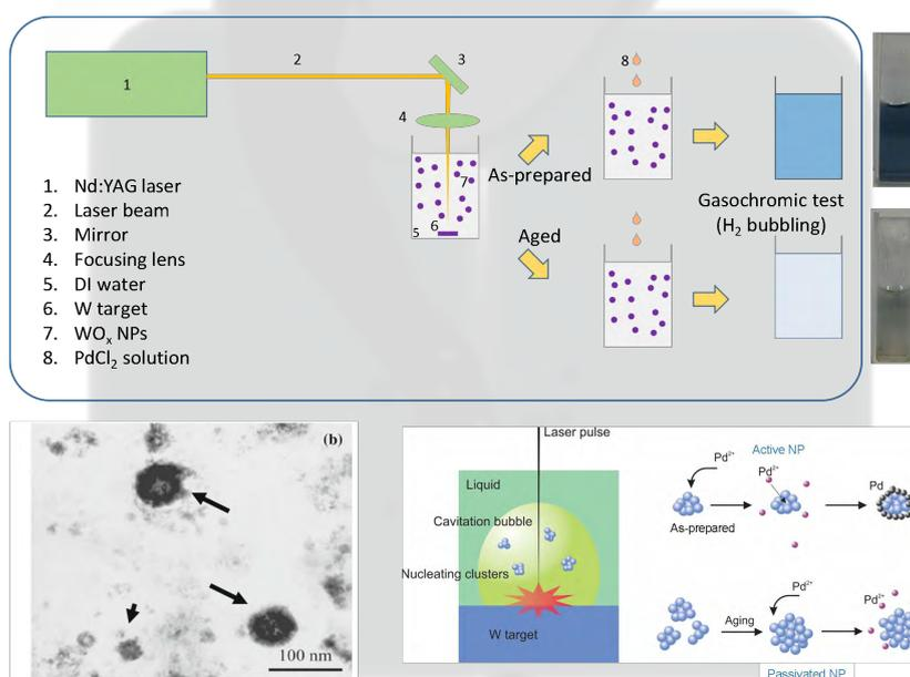
Figure 1 Laser assisted reduction process for synthesis of decorated LSPR materials  $\text{WO}_x$ . TEM images of  $\text{WO}_x@$ Pd (bottom left panel) core-shell structures. The other parts show the ability to detect hydrogen by these systems and the effect of resting time on core-shell structure formation.
