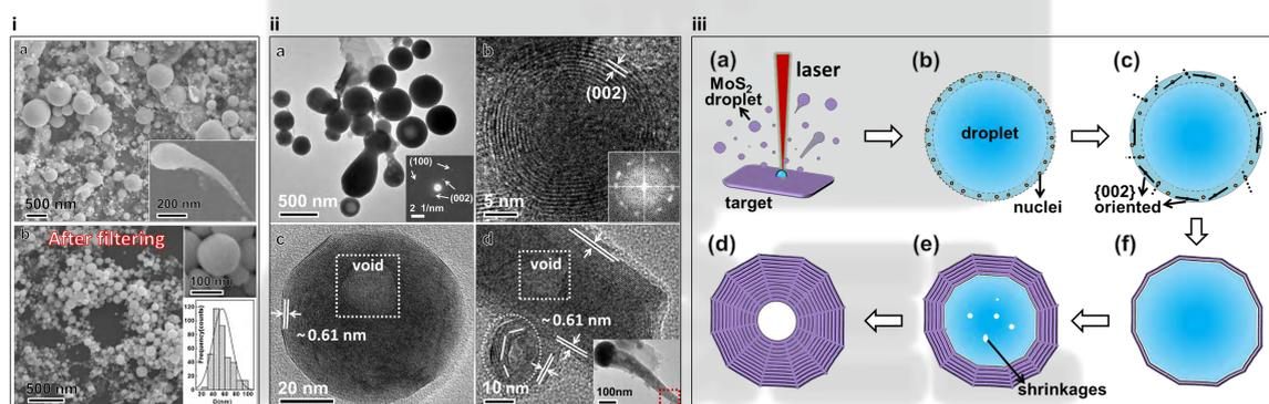
Figure 1 (i) Morphology, (ii) microstructure and (iii) growth mechanism of as-prepared MoS<sub>2</sub>.
