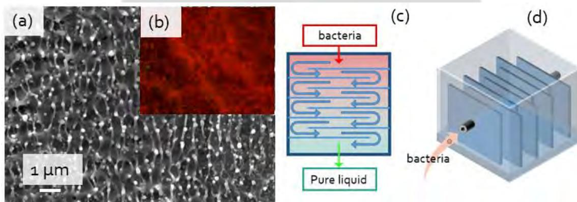
Figure 1. (a) SEM image of nanostructured Ti surface; (b) fluorescent photograph of the bacterial strains; (c) the upper view of flow-through filter and (d) its 3D model.
