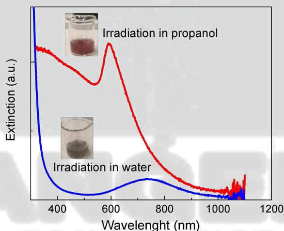
Figure 1 Typical plasmon resonances after the irradiation of colloidal copper nanoparticles in different liquid environments
