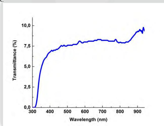
Figure 1 Transmittance of gold nanoparticles in solid sodium nitrate.
