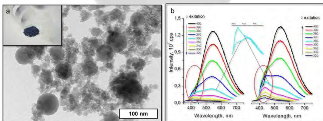
Figure 1 TEM image (a) and photoluminescence spectra (b) of TiO<sub>2</sub> powder.
