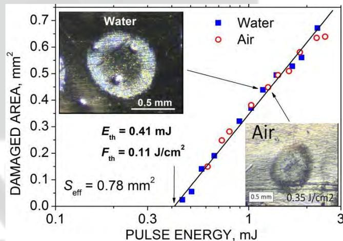
Figure 1 The area of the damage spots produced on the Sn surfaces in air and water as a function of laser pulse energy. The measured threshold energy, fluence and efficient spot area are indicated. The insets show optical microscope image of typical spots.
