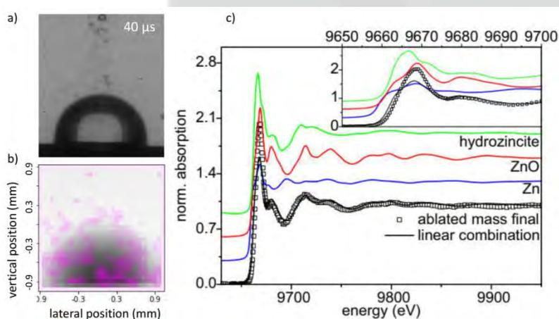
Figure 1: (a) Visible snapshot of the PLAL bubble at maximum extension at 40  $\mu$ s compared to (b) radiographic image overlaid with dark-field signal (pink). (c) XAFS spectrum of the final state of the zinc suspension after ablation compared to model functions of different chemical products [7].
