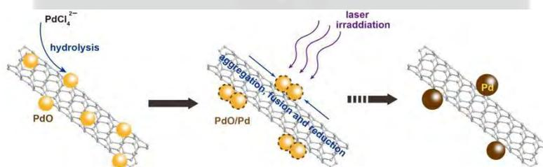
Fig. 1 Schematic illustration of the reduction of PdO to form Pd-PdO interface by laser irradiation.
