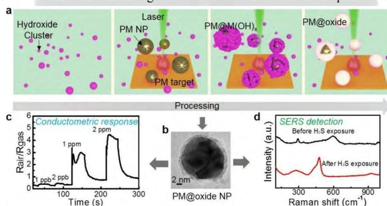
Figure 1 (a) The formation of the  $PM@oxide$  NPs, (b) a transmission electron microscopy image of a typical  $PM@oxide$  NP, (c) conductometric response of  $Au@SnO_2$  NPs to  $H_2S$  gas, and (d) SERS-based detection of  $H_2S$  with  $Au@CuO$  NPs.
