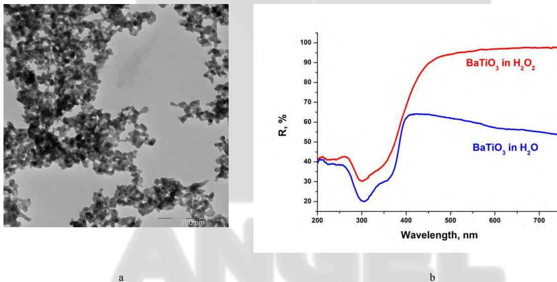
Figure 1. TEM view of NPs of BTO generated by ablation in H<sub>2</sub>O<sub>2</sub> at pulse duration of 200 ns. Scale bar denotes 200 nm (a). Reflectivity of BTO nanoparticles generated by laser ablation in H<sub>2</sub>O and H<sub>2</sub>O<sub>2</sub> (b) with respect to Al<sub>2</sub>O<sub>3</sub> ceramics.
