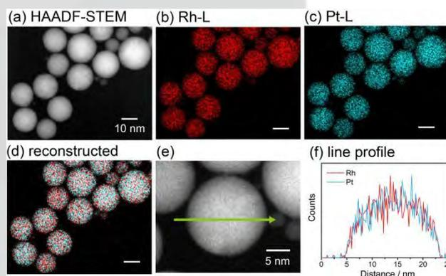
Figure 2 STEM-EDS mapping for the NPs fabricated in RhPt solution. (a) HAADF-STEM image, (b) Rh-L and (c) Pt-L STEM-EDS mappings, (d) reconstructed image, (e) magnified HAADF-STEM image of a particle in (a), and (f) line profile of Rh and Pt along the arrow in (e).
