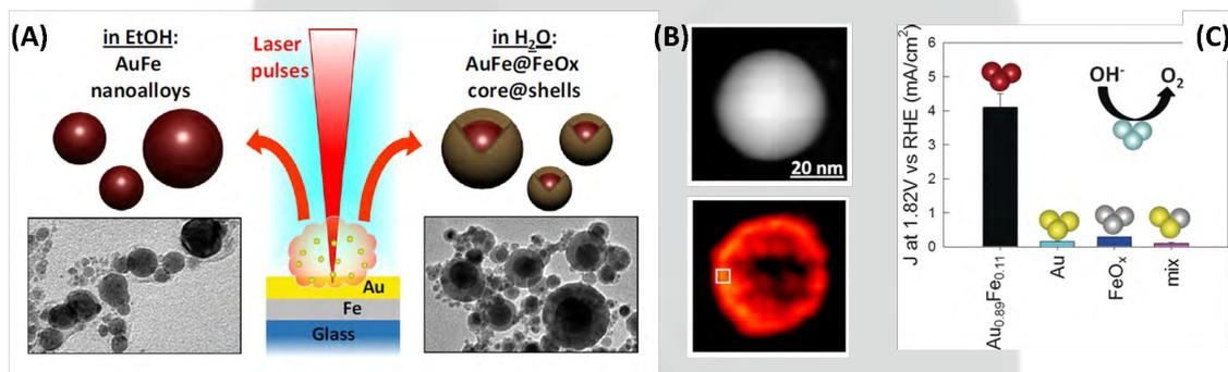
Figure 1. (A) Iron-rich Au-Fe nanoalloys are obtained in ethanol by nanosecond laser ablation of a bilayer Au/Fe film (left). When the same film is ablated in water, core-shell NPs of iron oxide-AuFe metal alloy (iron poor) are achieved.[8,9] These NPs possess interesting properties for photonics (B), exhibiting localized surface plasmons,[11] and for catalysis (C), with enhanced activity compared to single element analogues[10].
