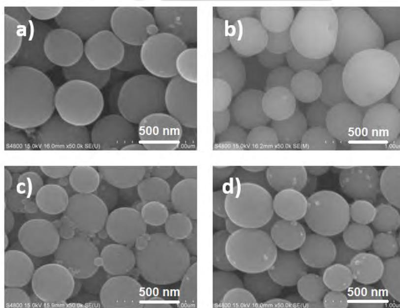
Figure 1 Images of nanoparticles and nanocomposites obtained by pulsed laser irradiation of  $\alpha$ -Fe<sub>2</sub>O<sub>3</sub> nanoparticles dispersed in different organic solvents: (a) toluene, (b) ethyl acetate, (c) acetone and (d) ethanol.
