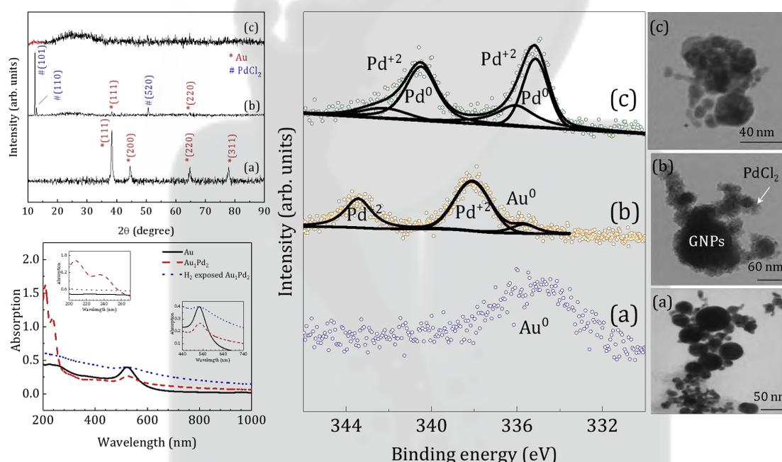
Figure 1 Left panel up: XRD, Left panel down: Absorption spectra of GNPs, Au<sub>1</sub>Pd<sub>2</sub> sample before and after hydrogen exposure, middle panel: XPS and right panel: TEM images of (a) GNPs, (b) Au<sub>1</sub>Pd<sub>2</sub> sample before and (c) after 10% H<sub>2</sub> exposure.
