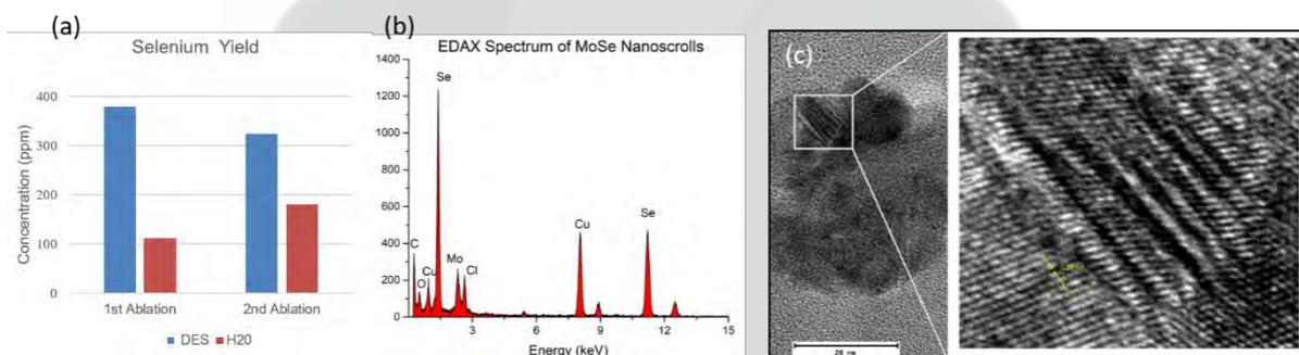
Figure 1. (a) Difference of the yield concentration in ppm of selenium present in MoSe<sub>2</sub> nanosheets synthesized in deep eutectic solvent (DES) and H<sub>2</sub>O. (b) EDS analysis of MoSe<sub>2</sub> nanosheets synthesized in DES showing a low oxygen existence, compared to the selenium peaks. (c) TEM image of MoSe<sub>2</sub>. Insert shows fringes indicating crystallinity.
