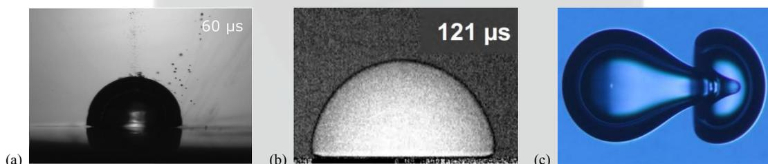
Figure 1 : Imaging of mm sized cavitation bubbles during laser ablation in liquids: (a) Shadowgraph image [2], (b) x-ray flash radiography [3]. Both imaging techniques are not well suited for investigating material synthesis inside the bubble.
