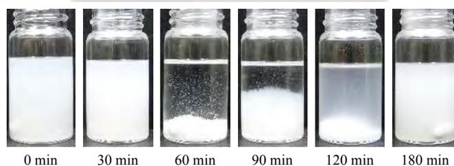
Figure.1 Temporal appearance change of CaO powder dispersed in ethanol during laser ablation.
