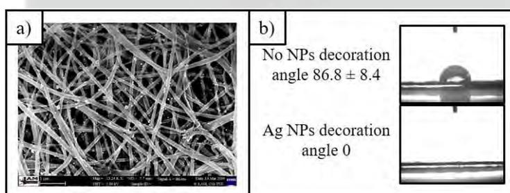
Figure 1 a) micrograph of the membrane decorated with the Ag NPs and b) contact angle test of the sample before and after the nanoparticle decoration, displaying that after the decoration, the membrane becomes hydrophilic.
