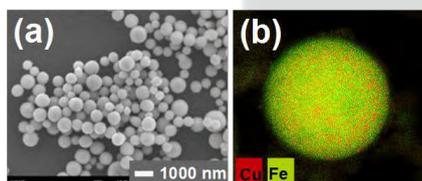
Figure 1 SEM image (a) and EDS elemental mappings (b) of CuFe particles obtained by pulse laser irradiation of Cu and Fe<sub>3</sub>O<sub>4</sub> nanoparticles dispersed in ethanol. Conditions of laser irradiation 532nm, 170 mJ/impuls cm<sup>2</sup>, 1h.
