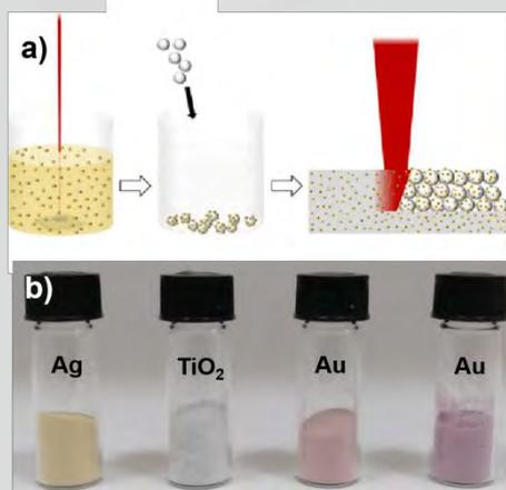
Figure 1. a) Scheme of the proposed methodology for laser generated nanoparticles supporting on polymer powders and the subsequent PBF-LB processing. b) Examples of a polymer powder after supporting of different laser generated nanoparticles.
